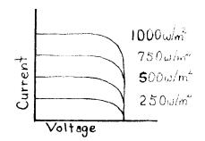
The power output of a silicon PV device decreases with increasing temperature. The current of the device increases slightly with temperature, but the voltage decreases at a more rapid rate. The result is a decrease in power of 0.4-0.6 percent per degree C.
