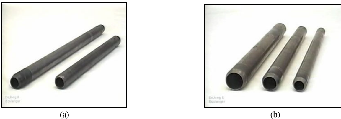
Figure 3-7. Split-Barrel Samplers: (a) Lengths of 457 mm (18 in) and 610 mm (24 in); (b) Inside diameters from 38.1 mm (1.5 in) to 89 mm (3.5 in).
