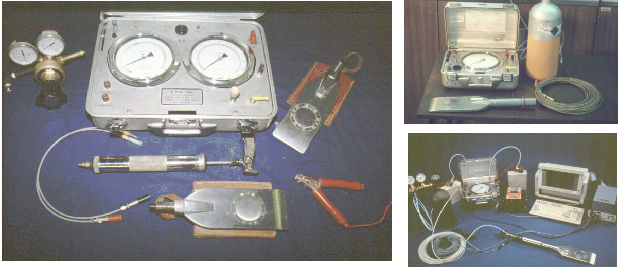
Figure 5-16. Flat Plate Dilatometer Equipment: (a) Modern Dual-Element Gauge System; (b) Early Single-Gauge Readout; (c) Computerized Data Acquisition Model.
