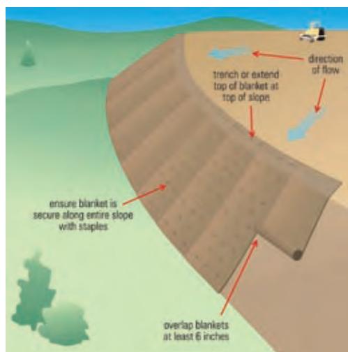
Figure 9. Illustration of erosion control blankets installed on slope.
