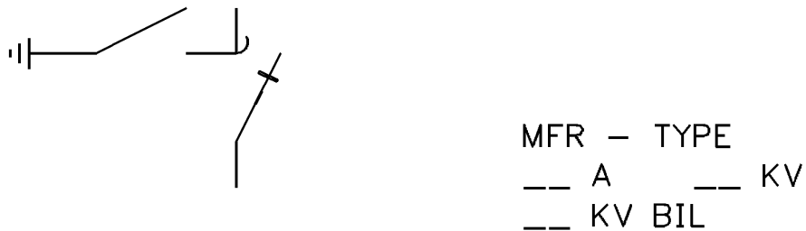
Figure 3-6: Three-Phase Gang-Operated Disconnecting Switch with Horn Gaps and Grounding Switch. Ref. IEEE Std. 315. Figs. 4.6.1, 4.6.6, and 3.9.1. Copyright © 1975. IEEE. All rights reserved.
