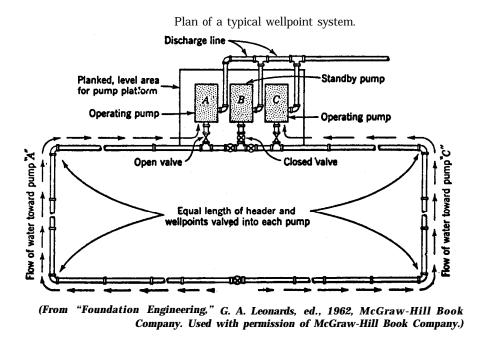
Figure 5-1. Plan of a typical wellpoint system.
