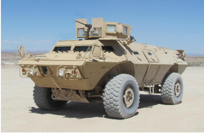
Figure 1. Mobile Strike Force Vehicle Armored Personnel Carrier (Photo by Textron Marine and Land Systems)
