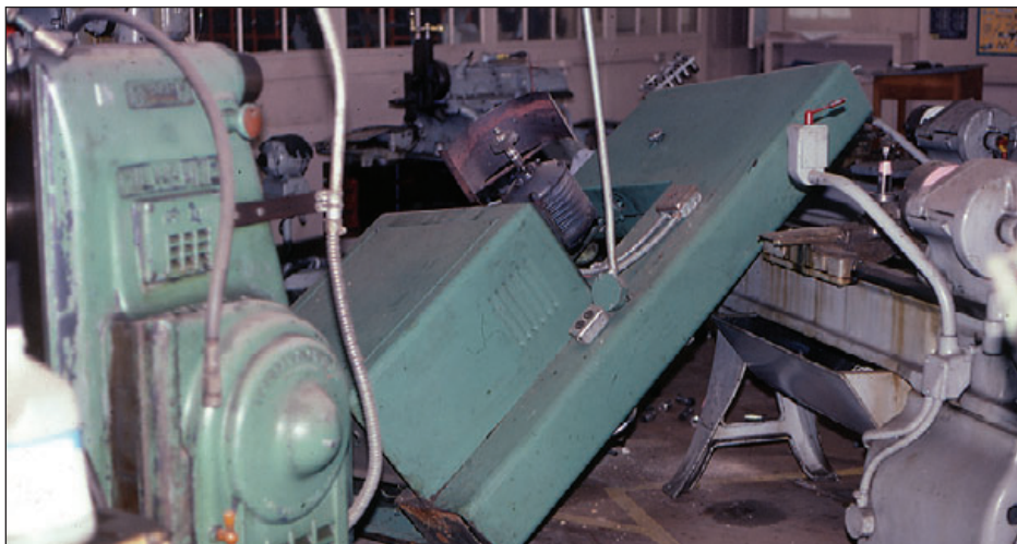
Figure 4-9: Fallen shop equipment, Coalinga, CA, 1983
