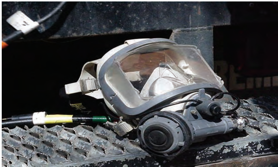
Figure 11.3.31 Full Face Lightweight Diving Mask with Communication System
