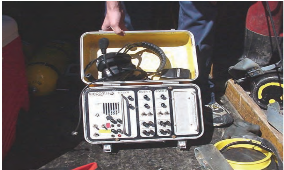
Figure 11.3.36 Communication Box System
