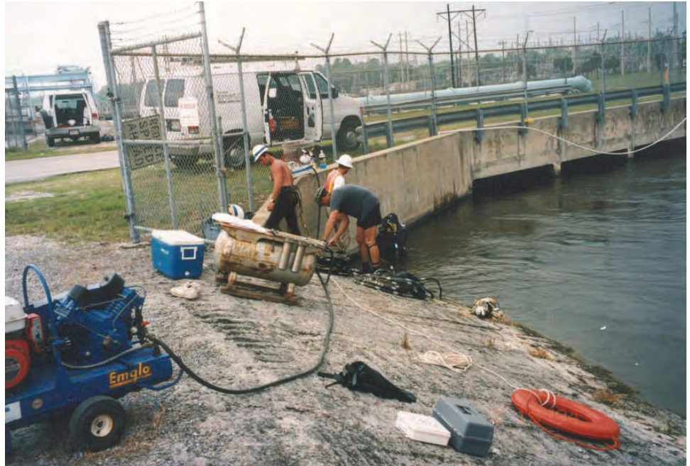
Figure 11.3.32 Surface-Supplied Air Equipment, Including Air Compressor, Volume Tank With Air Filters, and Umbilical Hoses
