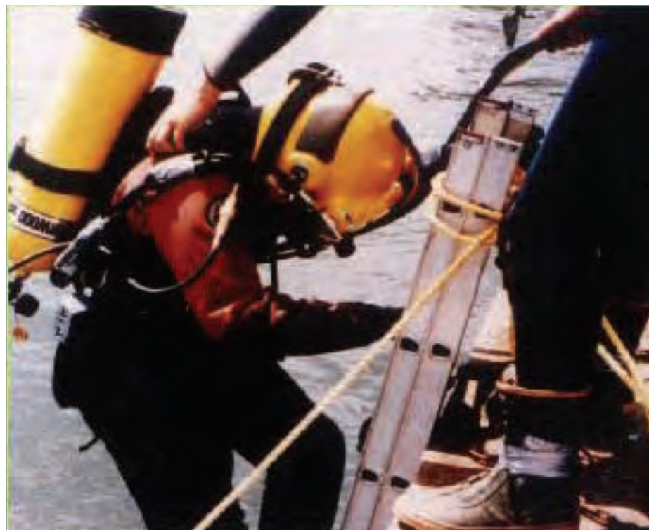
Figure 11.3.35 Surface-Supplied Diver with a Reserve Air Tank
