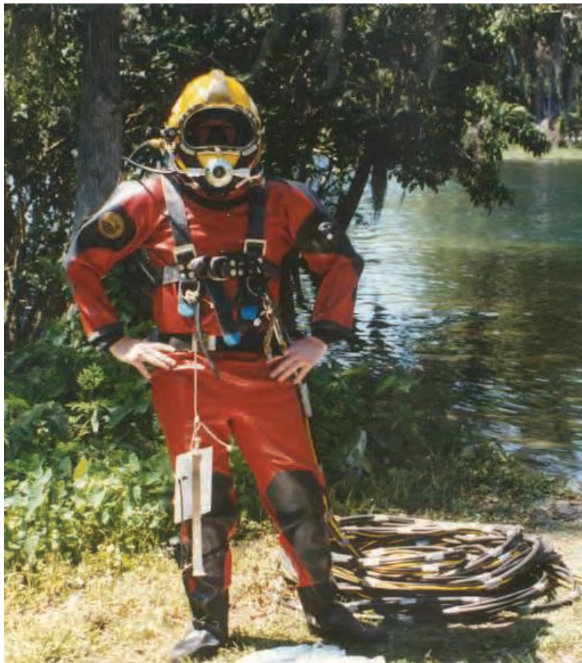
Figure 11.2.23 Surface Supplied Air Diving Equipment
