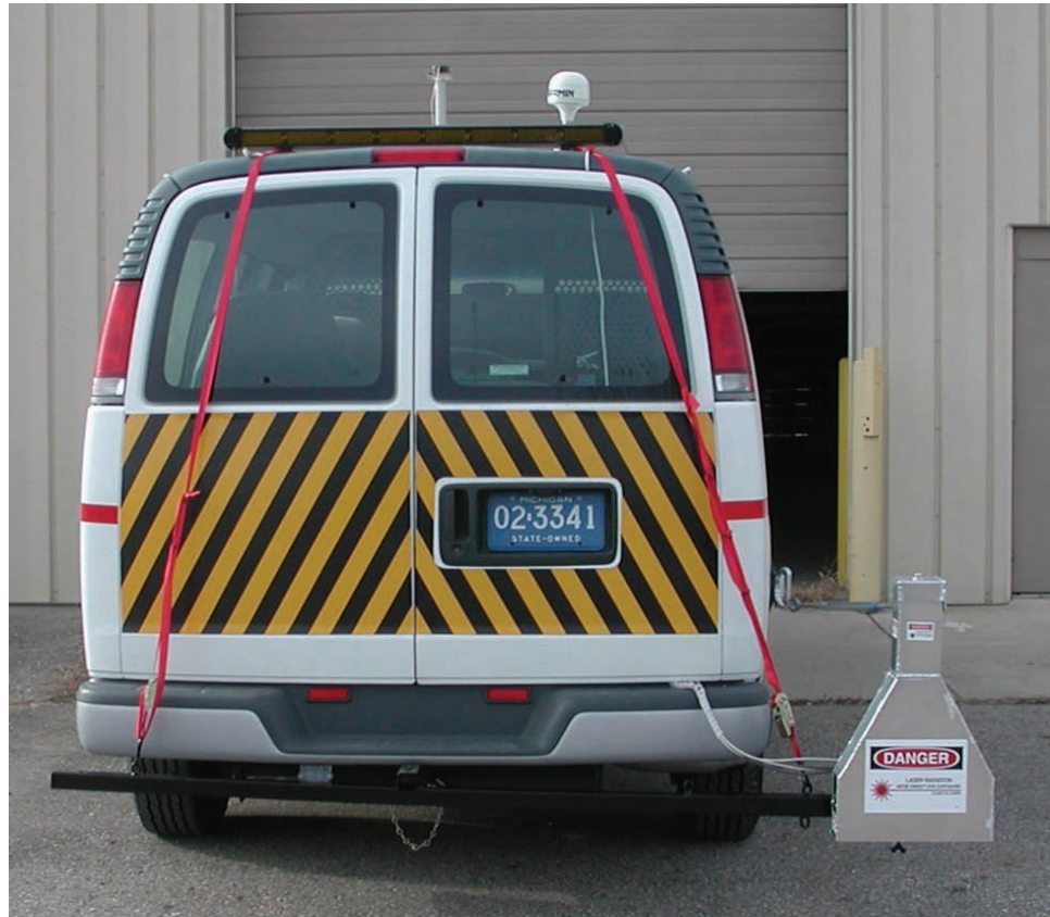
Figure 3.4.9 High Speed Underclearance Measurement System
