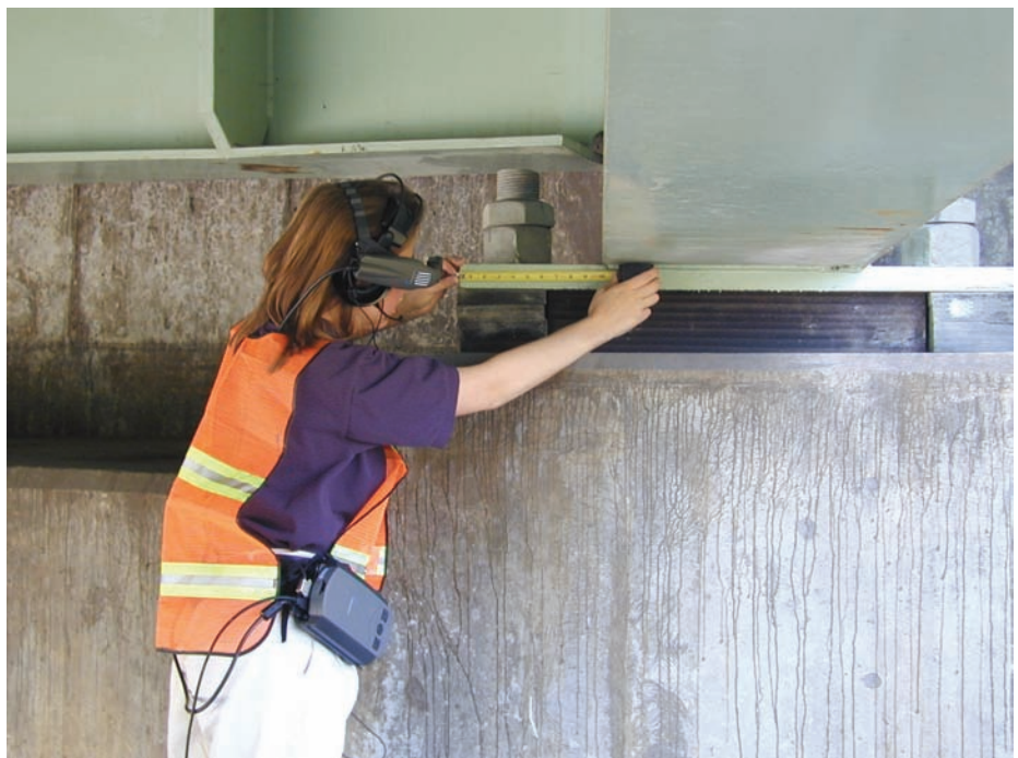
Figure 4.1.6 Inspector Using Wearable Computer
