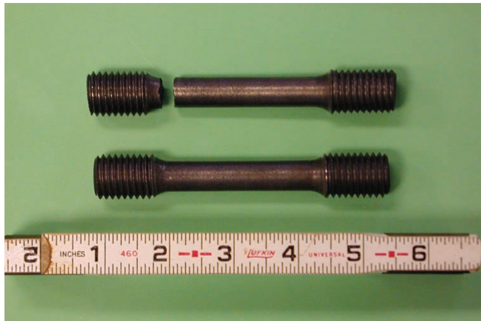
Figure 8.1.9 Brittle Fracture of Cast Iron Specimen
