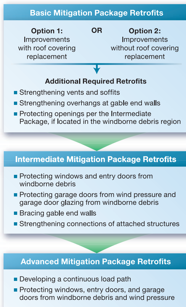
Figure 15-15. Wind Retrofit Mitigation Packages
