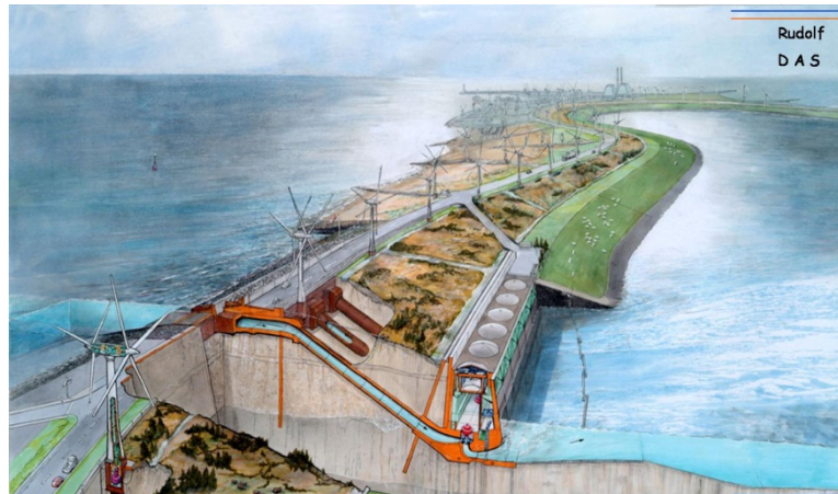
Figure 6. Cross section of Energy Island PSH.
