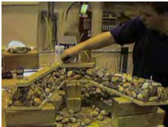
Figure 58. Photo. Fabrication of the cross vane.
