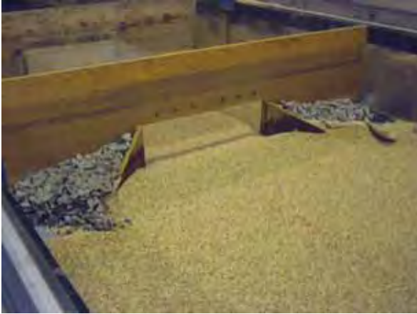
Figure 26. Photo. 45-degree inlet wingwalls before scour.
