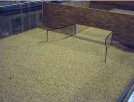
Figure 33. Photo. Elongated, streamlined wingwalls before scour.
