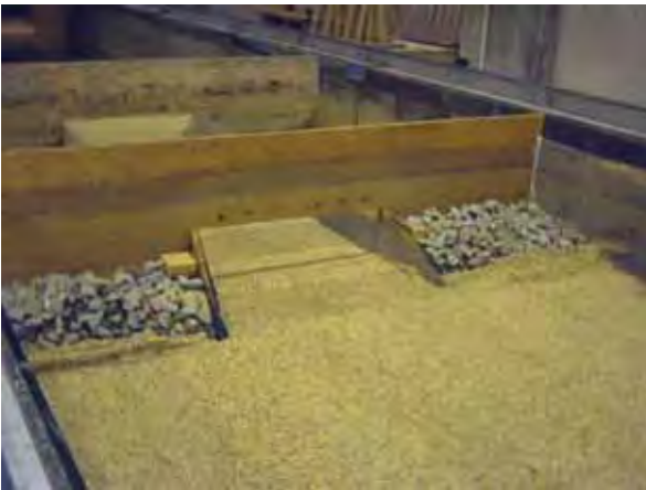
Figure 28. Photo. 8-degree inlet wingwalls before scour.
