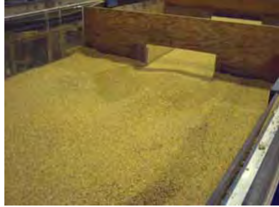
Figure 32. Photo. Truncated, circular wingwalls after scour.
