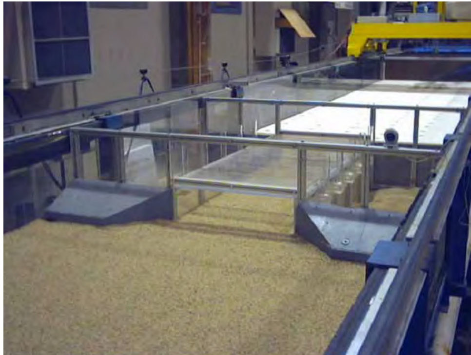
Figure 19. Photo. Outlet prior to scour test.
