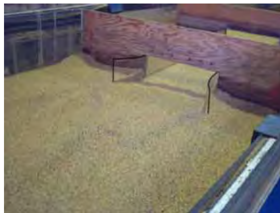
Figure 35. Photo. Short, streamlined bevel wingwalls after scour.
