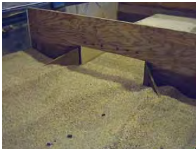
Figure 40. Photo. 45-degree wingwalls after scour.
