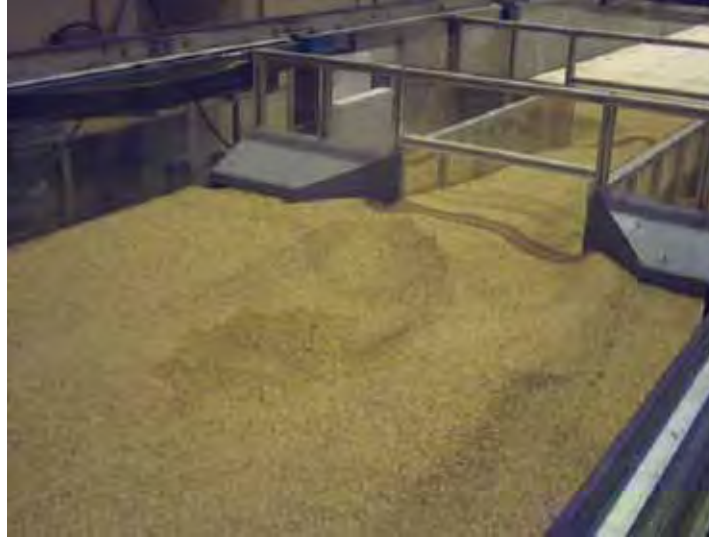
Figure 25. Photo. Outlet scour after test.
