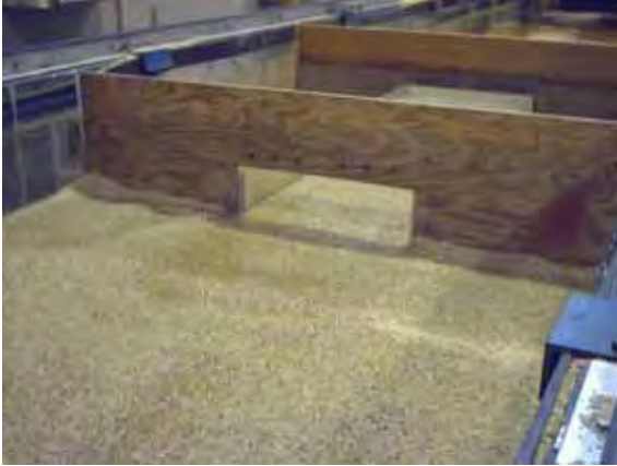
Figure 31. Photo. Truncated, circular wingwalls before scour.
