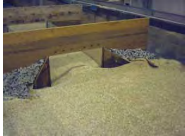
Figure 27. Photo. 45-degree inlet wingwalls after scour.
