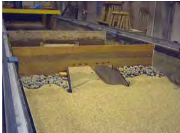
Figure 29. Photo. 8-degree inlet wingwalls after scour.
