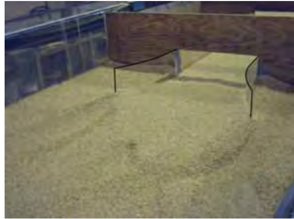
Figure 34. Photo. Elongated, streamlined wingwalls after scour.
