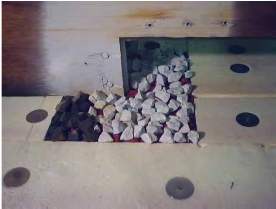
Figure 3. Photo. Riprap test for a rectangular culvert.
