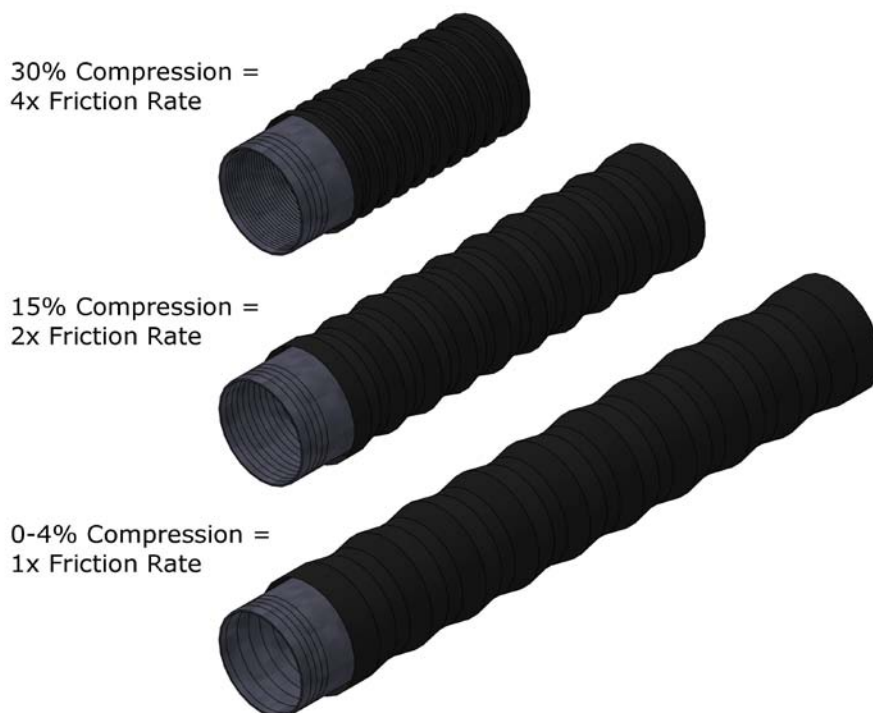
Figure 3. Increased friction rate in compressed flexible duct
