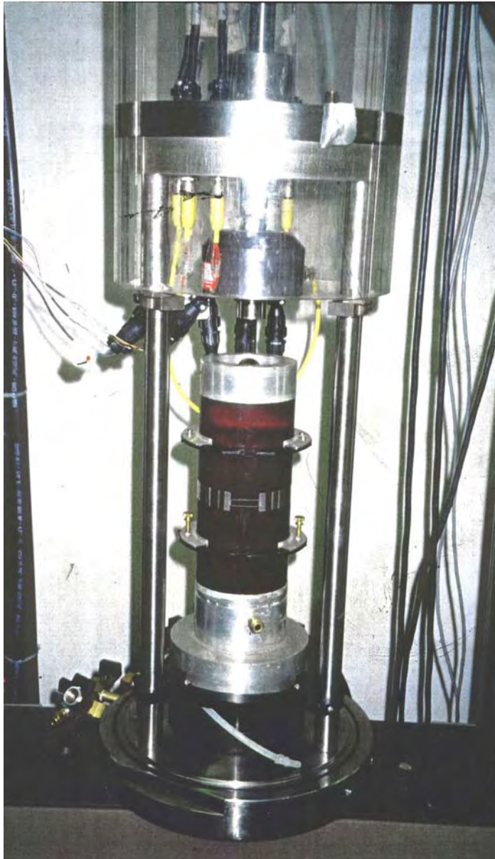
Figure 5-16. Triaxial cell set-up for resilient modulus test.
