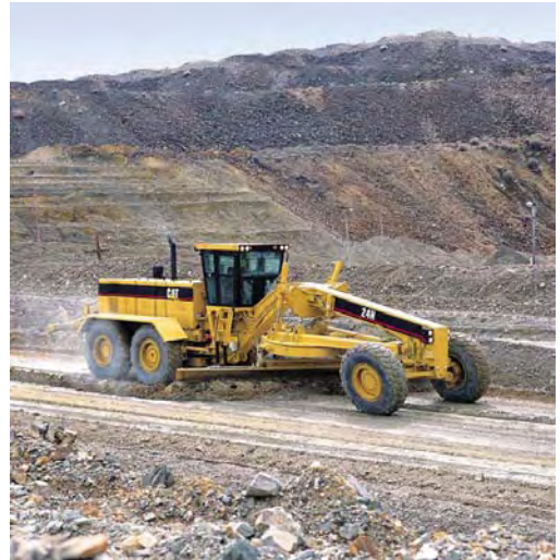
Figure 8-9. Motor grader (photo courtesy of Caterpillar)
