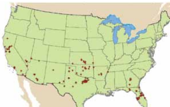
b) Fossil-fired power plant sources of CO 2 within 20 miles of municipal wastewater facilities in the preferred climate region
