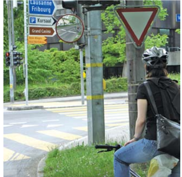
Figure 25. Convex mirrors improve bicyclist visibility for drivers of large or high-profile vehicles in Bern, Switzerland. (Note: photo taken from vantage point of motorist at stop line.)
