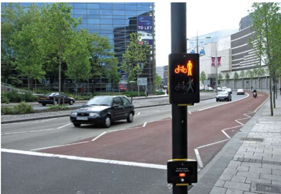
Figure 10. Near-side pedestrian signal with confirmation light in Bristol, United Kingdom.
