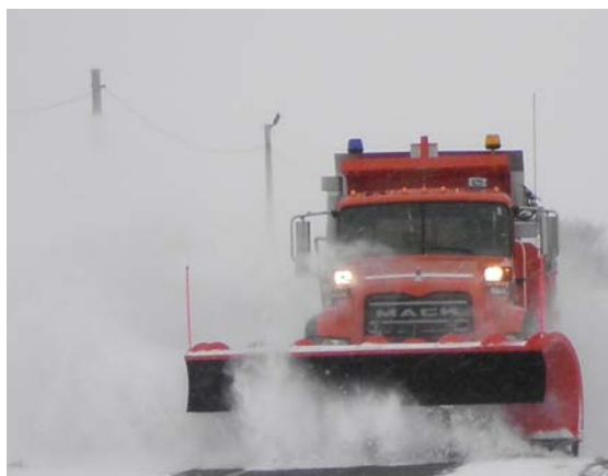
Figure CO-1. Truck with 14 ft. wide front plow.
