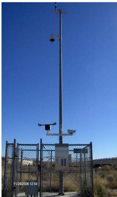
Figure AZ-1. Visibility sensor in ADOT DUST warning system.
