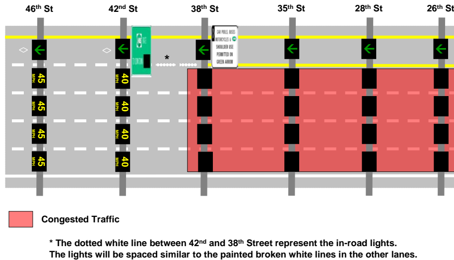
Figure MN-7. Striping and signing with PDSL open.
