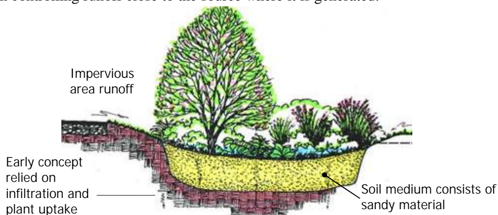
Figure 1.1 Bioretention facility Conceptual Cross-sectional Layout (early design)
