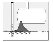
When installed and operated according to the manufacturer's instructions, a groundwater monitoring system meets the federal leak detection requirements for USTs. Operation of a groundwater monitoring system at least once each month fulfills the requirements for the life of a tank. Groundwater monitoring can also be used to detect leaks in piping (see the section on leak detection for piping starting on page 22).
