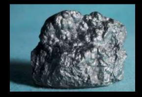
Lead's surface is greyish, but after scratching or scraping it, you can see that the actual color of the metal is white. Because it is soft, lead is used as backing material when punching holes with a hollow punch or when forming shapes by hammering copper sheets.
