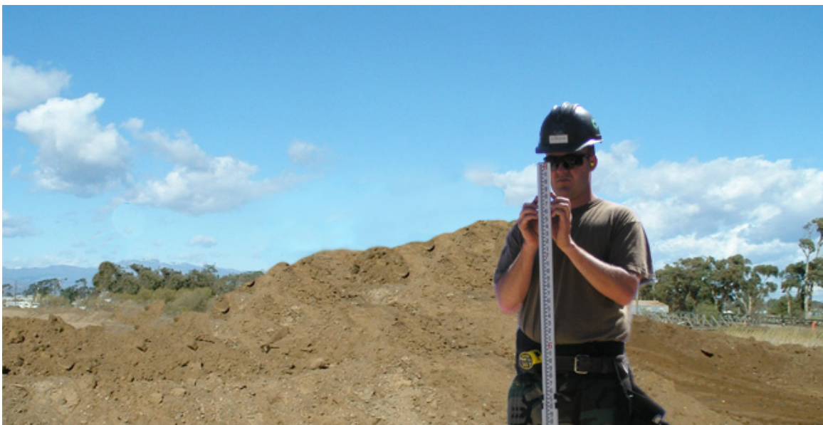
Figure 4-7 Laser level rod equipped with a laser detector.
