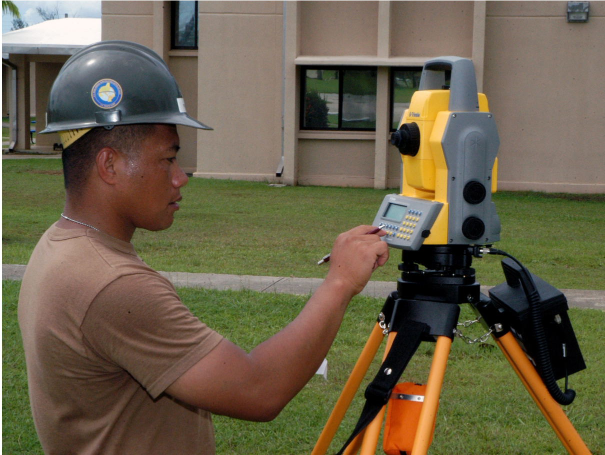
Figure 4-3 – An electro-optical distance measuring instrument (Geodimeter).
