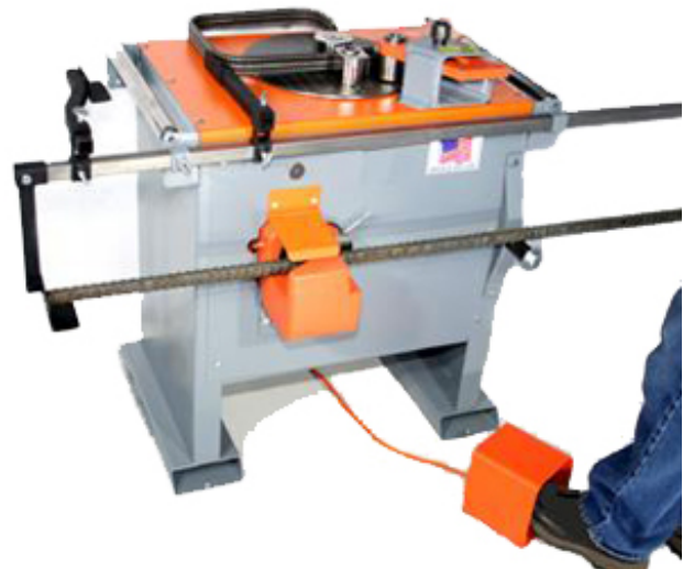
Figure 3-14 — Table cutter and bender.
