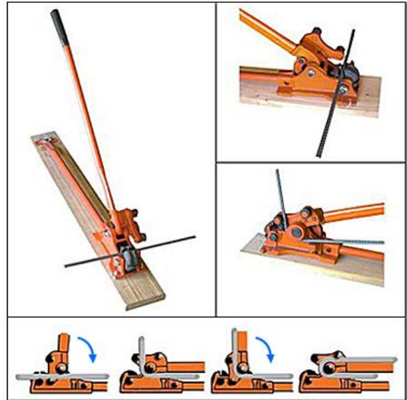
Figure 3-11 — Manual cutter and bender.
