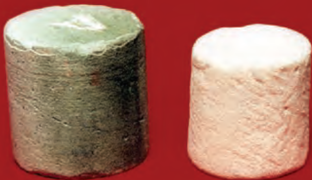
In the presence of CO 2 and hence carbonic acid, ThermaLock (left) remains unaffected for a long time, while Portland cement (right) quickly degrades.
