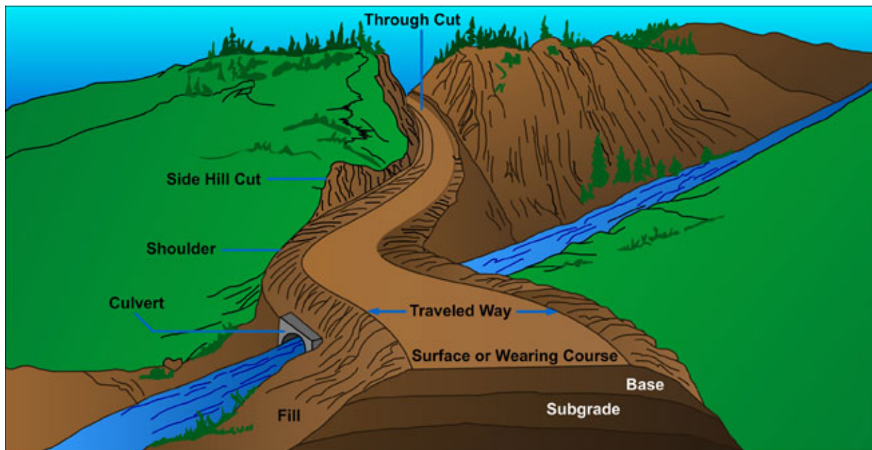
Figure 7-1 — Perspective view of road with road nomenclature.
