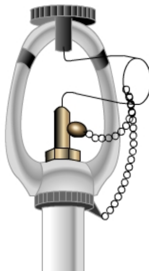
Figure 4-10 — Sprinkler pre-prime plugs.
