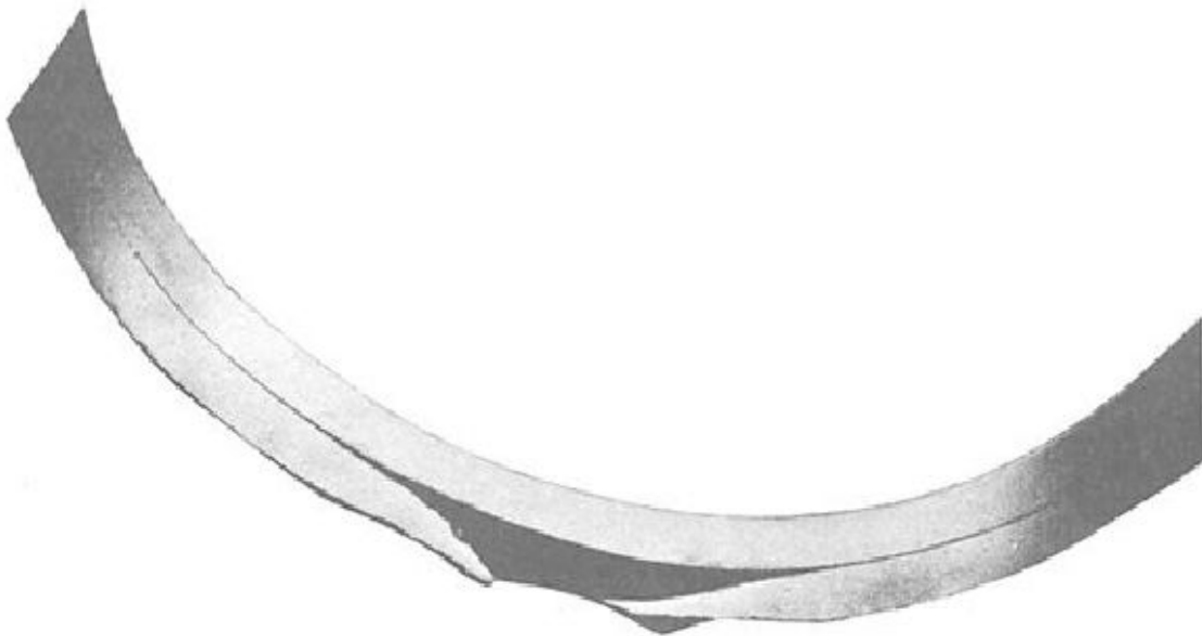
Figure 8-22 — Lamination of a tube wall (fabrication defect).
