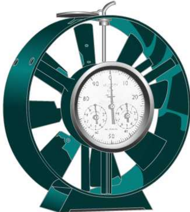
Figure 9-8 — Rotating vane anemometer.
