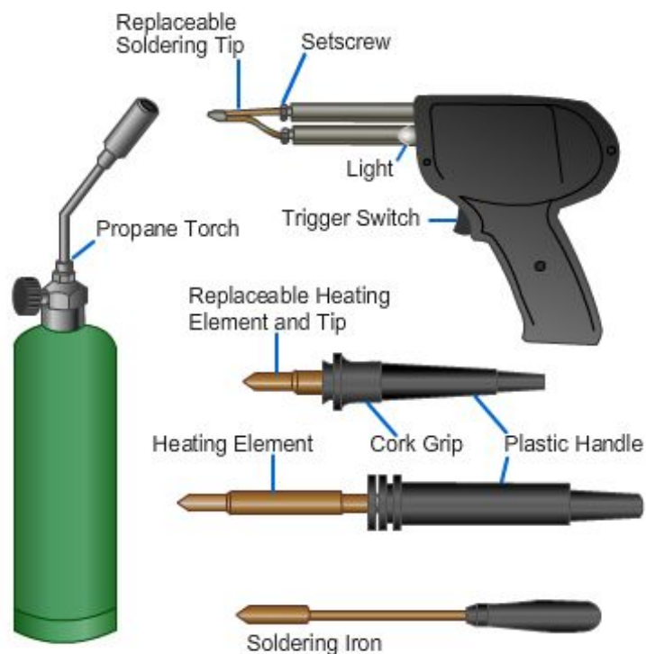
Figure 8-119 – Sources of heat for soldering splices.
