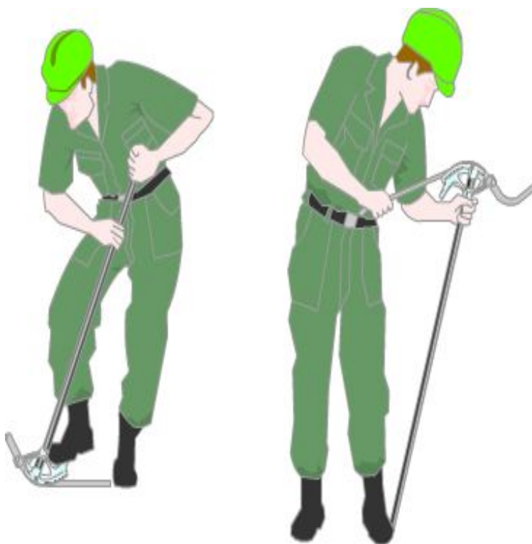
Figure 8-63 – Bending on the floor and in the air.
