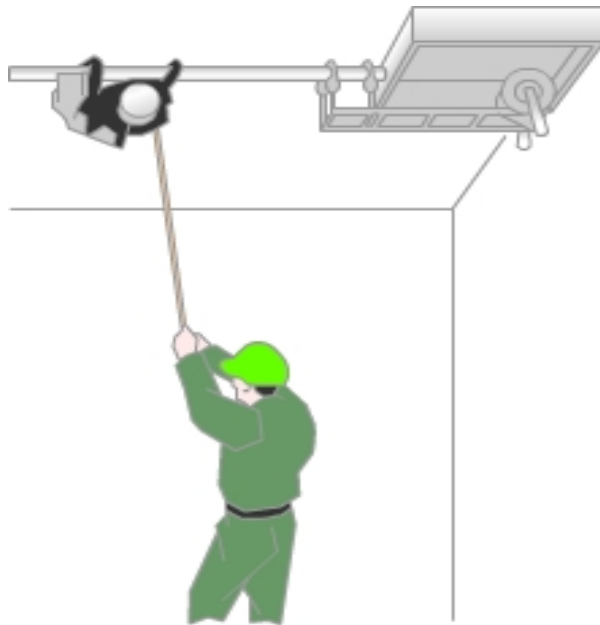
Figure 8-79 – Pulling in an overhead pull box with the puller mounted independently for extra cable.
