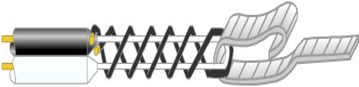
Figure 8-73 – Wires attached to fish tape.
