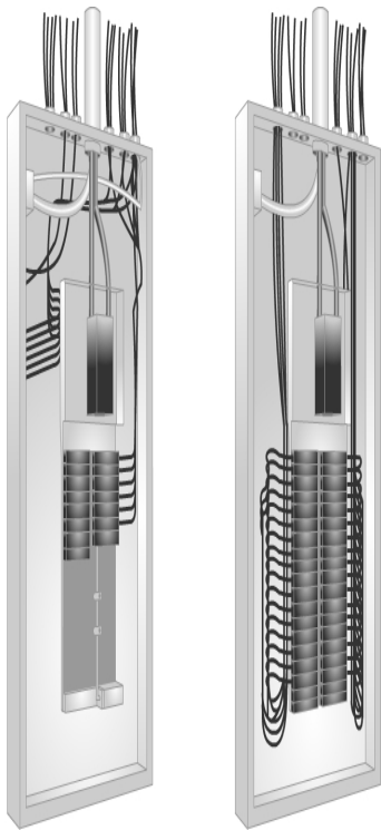
Figure 8-86 – Panelboard connections without excess wire.
