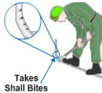
Figure 8-66 – Bending with a hickey using small bites.
