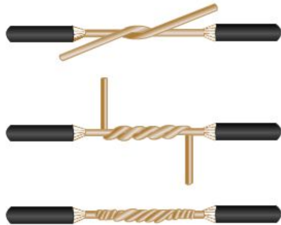
Figure 8-115 – Western Union splice used where substantial strain may be placed on the connection.
