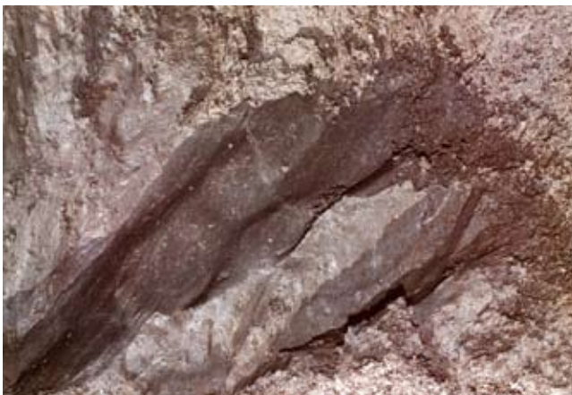
Figure TS14A–19 Slickensides in exposure of clay soil
