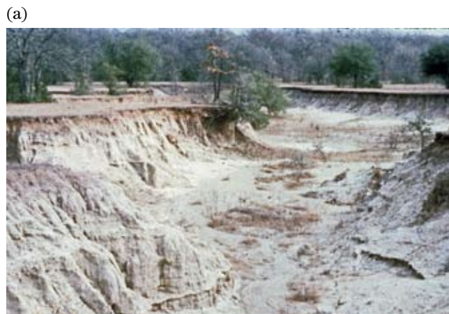
Figure TS14A–24 Photographs of exposure of dispersive clays in streamside slopes in TX and OK
