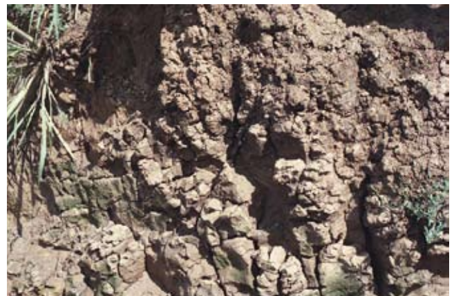
Figure TS14A-23 Blocky structured clay in streambank exposure
