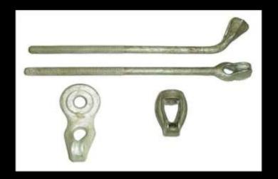
**Thimble eye washers** - are stout washers forged with a thimble eye at a 45 degree angle for use with down guys and sidewalk guys. Install the thimble eye washer under a nut, making sure you tighten the nut down snugly.
