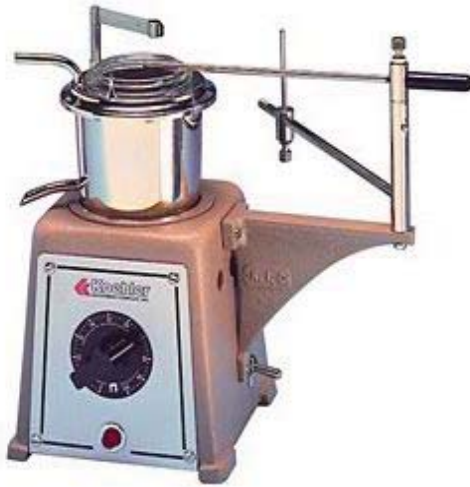
Figure 10-38 – Example of a Tag open-cup flash point tester.
