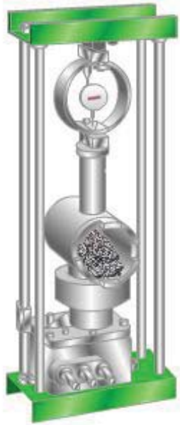
Figure 10-44 – Marshall stability testing head mounted in CBR jack.
