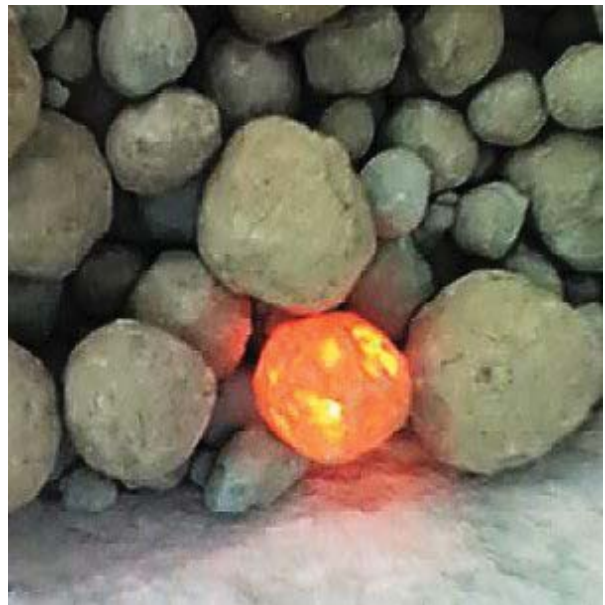
Figure 10-16 — Example of clinkers.
