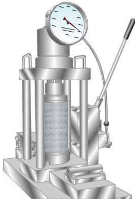
Figure 10-27 — Typical compression testing machine.
