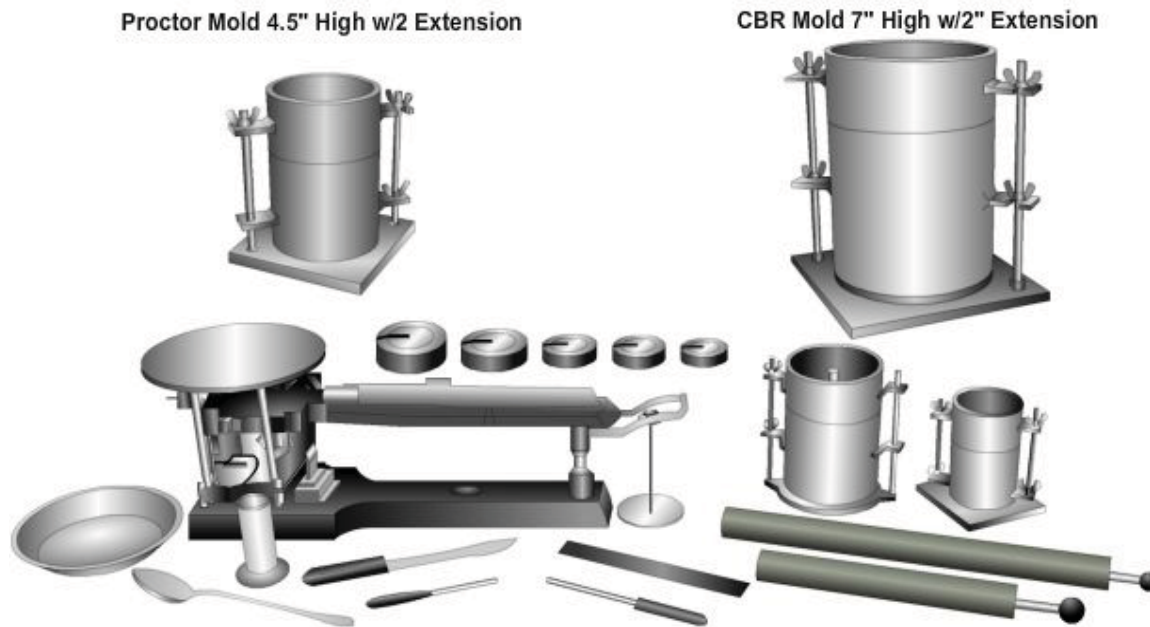
Figure 10-1 — Typical soil compaction testing apparatus.
