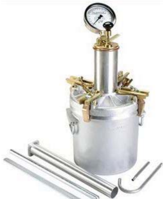
Figure 10-25 — Example of air-content test kit.
