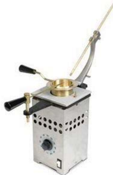
Figure 10-39 – Example of a Cleveland open-cup flash point tester.
