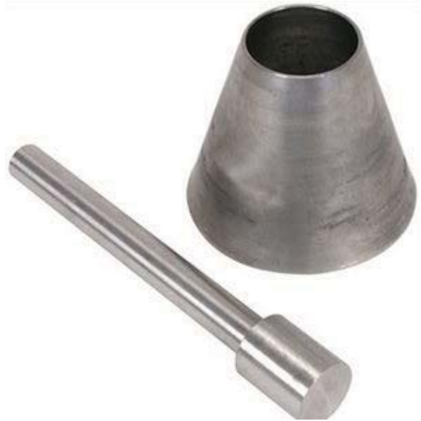
Figure 10-20 — Example of water-absorption cone and tamper.
