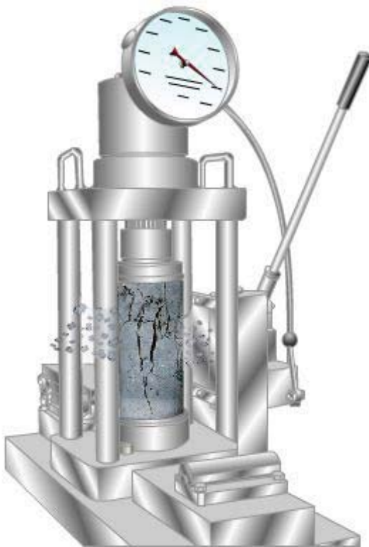
Figure 10-28 — Typical compression test cylinder fracture.
