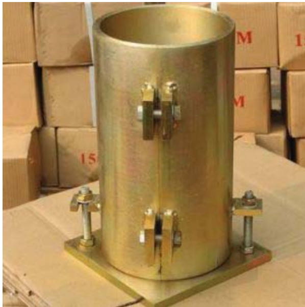
Figure 10-26 — Typical concrete cylinder mold.
