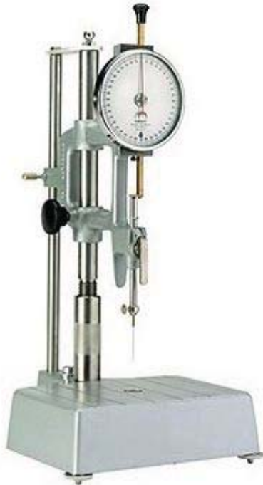
Figure 10-40 – Example of an asphalt penetrometer.
