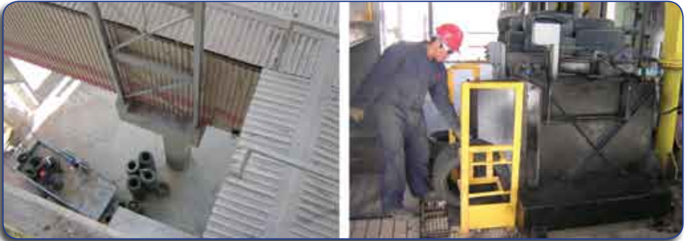
Exhibit 4-5. Tire metering systems for kiln introduction Photo courtesy of Terry Gray, TAG
