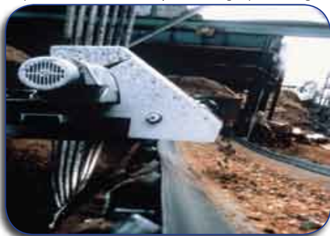
Conveyor belt to introduce wood and TDF into boiler system Photo courtesy of Terry Gray, TAG
