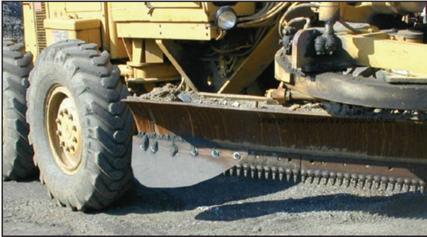
Figure 4.18—Homemade ditch cleaner for a grader.
