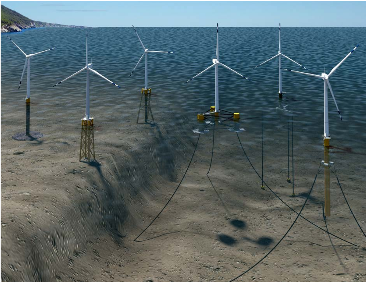
Figure 3.3. Six different offshore wind substructure types. The three on the far left are fixed-bottom substructures (monopile, jacket, and inward battered guide structure [also known as a twisted jacket]), and the three on the right are floating substructures (from left: semisubmersible, tension leg platform, and spar). Illustration by Josh Bauer, NREL
