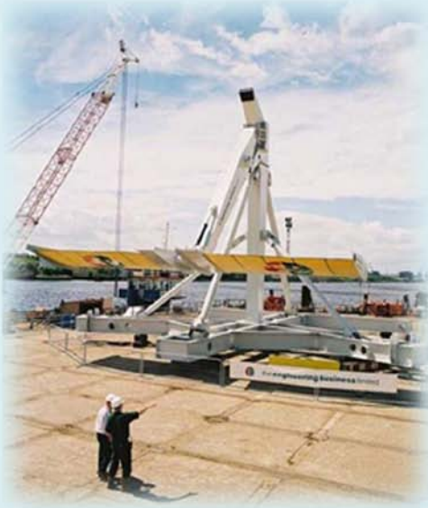
Oscillating Hydrofoil (Stingray) Source: The Engineering Business
