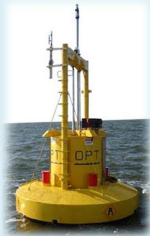
Point Absorber (PowerBuoy) Source: Ocean Power Technologies
