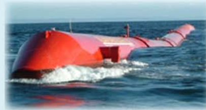
Attenuator (Pelamis) Source: Pelamis Wave Power
