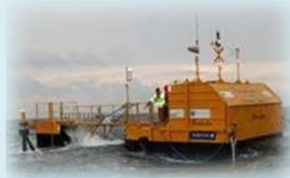
Oscillating Water Column (OEBuoy) Source: Ocean Energy
