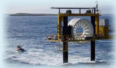
Ducted Horizontal Axis Turbine (Open-Centre Turbine) Source: OpenHydro
