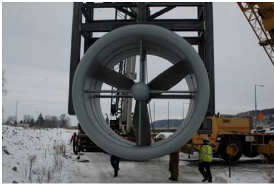
Figure 3-20. Ducted horizontal axis hydrokinetic turbine. Source: Hydro Green Energy LLC.
