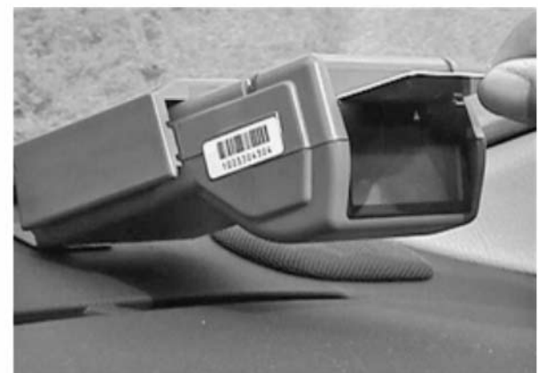
Figure 15. In-vehicle units (six types are available based on vehicle classification) with prepaid stored-value smart cards are required in every motor vehicle, including motorbikes, registered in Singapore.
