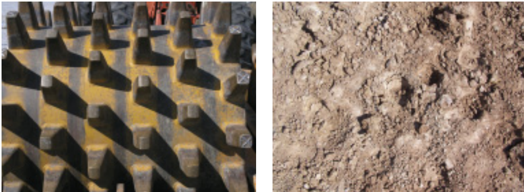
Figure 5.3: Sheepsfoot rollers compact soil.
