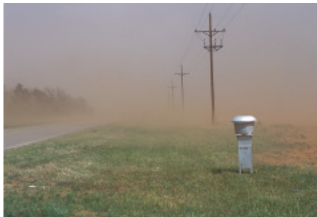
Figure 3.14: A dust cloud along a highway. Windblown particles are measured by the meter in the foreground.
