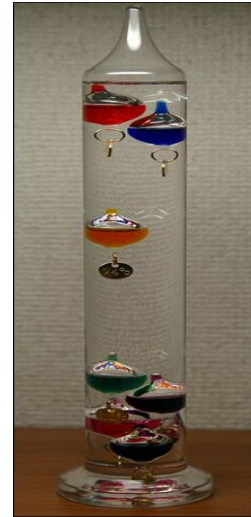
Galileo thermometer (the middle float shows the temperature) Image source: Wikipedia
