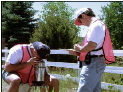
Surveyors using a Worden relative gravimeter Image source: New Mexico Tech
