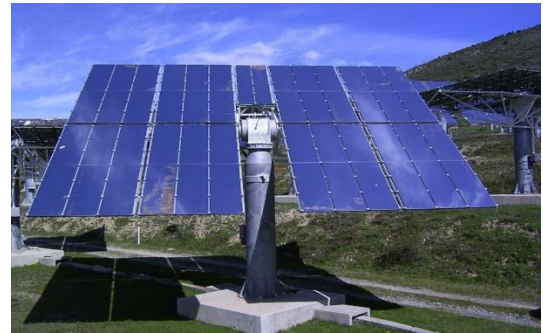
Heliostat Mirror Unit Image Source: en.wikipedia.org
