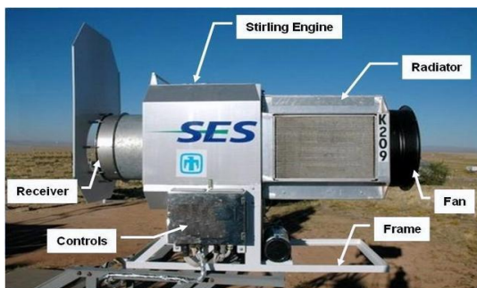
Receiver and Stirling Engine Assembly Image source: mtholyoke.edu
