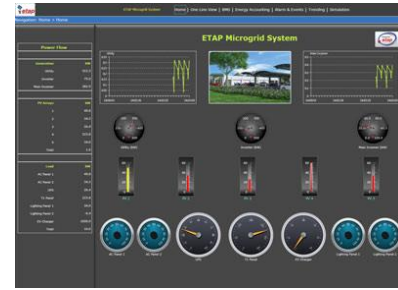
HMI display for a Microgrid control system
