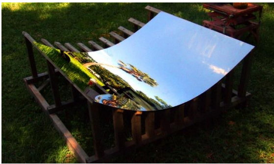
Laser Polished Stainless Steel on a Wooden Slat Support Frame Image Source: greenpowerscience.com
