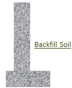
At-Rest Case No Wall Movement
