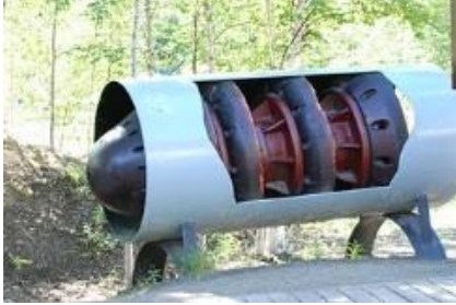
Pipeline Pig used for Cleaning and Inspections (Has a cutaway section for interior viewing)
