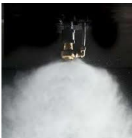
Water Misting Nozzle Image Source: nfpa.org
