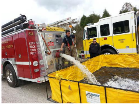
Tanker Truck dumping Firefighting Water into a Fold-up Holding Tank
