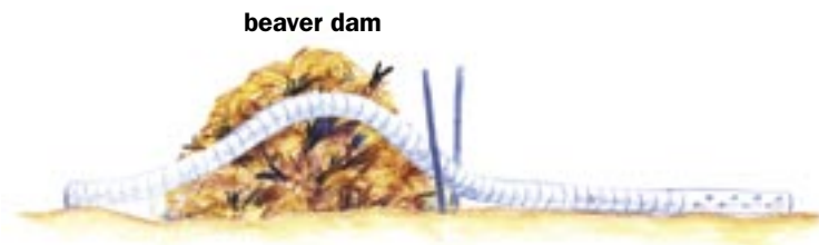
Figure 5-12. Massachusetts Beaver Pond Leveler
