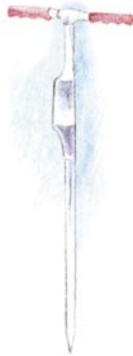
Figure 6-10. Effective baiting with a bait dispenser requires accurately finding the pocket gopher burrow. Use the probe to detect the main burrow, which is usually on the plug-side of the mound, 8-18 inches away from the plug (USDA, 1994).
