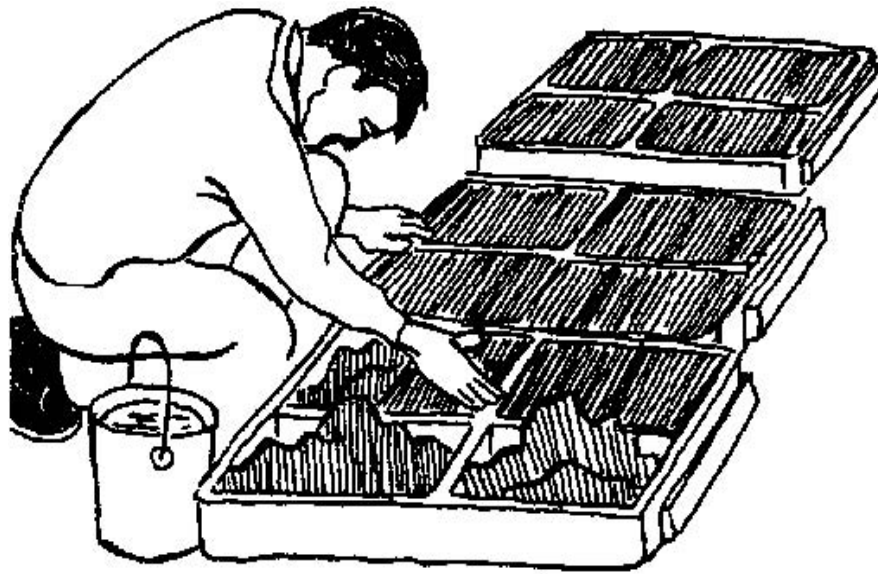
Figure 40. Kneading and leveling the blocks
