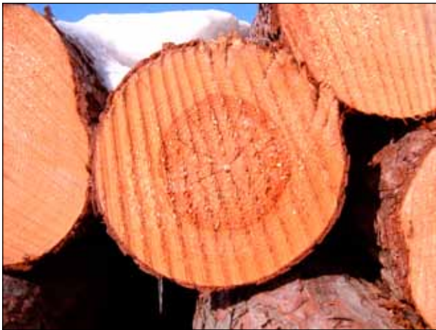
Figure 13-9. End checking in red pine logs.
